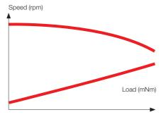
A special feature of the LSB 90 is the enormous force or very constant speed – even under high load – which allows a uniform grinding pattern.
